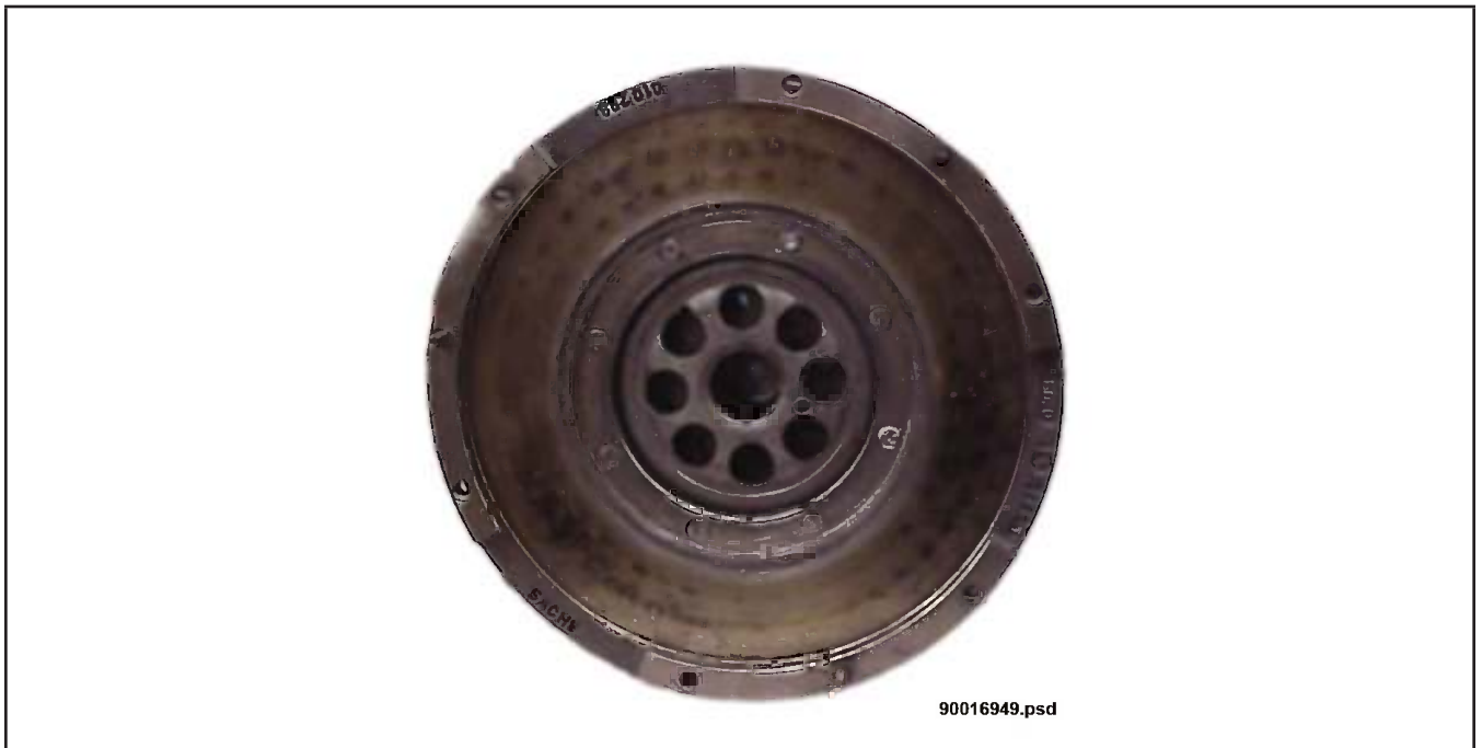
Figure 49 Dual Mass Flywheel Rear View (Clutch Disc Side, PT)
